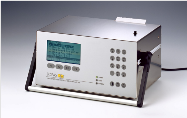
Clean Room Particle Counter LAP 340
